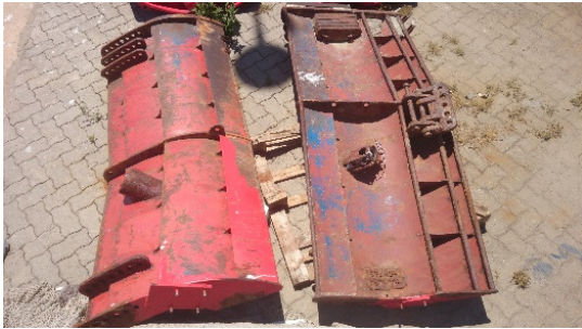
Figure 5. Example of a low-contact otter board model (Thyboroon T15VF) used in the 2013 study in Palamós.
